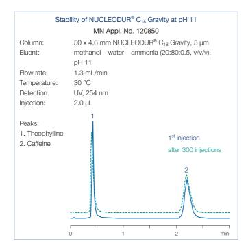
Even after 300 injections no loss of column efficiency - identified, e.g., by peak broadening or decrease in retention times - could be observed.
