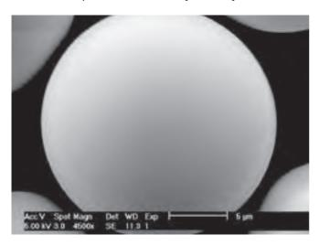
NUCLEODUR® silicas are synthesized in a unique and carefully controlled manufacturing process which provides silica particles, which are totally spherical. The picture shows the outstanding smoothness of the NUCLEODUR® surface.
