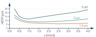
Column 50 x 4.6 mm, acetonitrile - water (50:50, v/v), analyte toluene
