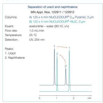
More polar compounds will have stronger interaction with the stationary aqueous layer than less polar compounds - resulting in a stronger retention. Nonpolar compounds exhibit faster elution profiles due to minor hydrophobic interactions. In the separation of uracil and naphthalene the elution order is guite often inverse on HILIC columns compared to RP columns.
