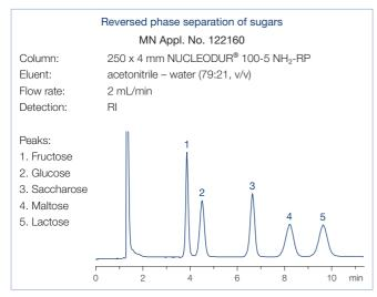
NUCLEODUR® NH2, too, belongs to the so-called multimode columns. It can be used for RP chromatography of polar compounds such as sugars in aqueous-organic eluent systems, for NP chromatography of substituted aromatics or chlorinated pesticides with organic mobile phases such as hexane, dichloromethane or 2-propanol, but also for ion exchange chromatography of anions and organic acids using conventional buffers and organic modifiers.
