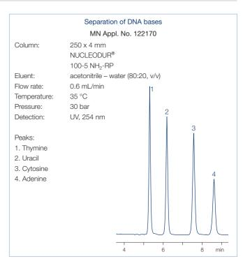
Based on superspherical NUCLEODUR® this phase features a high pressure stability, which makes it the perfect choice for preparative separations as well as for LC/MS. Additionally, the high batch-to-batch reproducibility of NUCLEODUR® NH2 enables reliable analyses especially for routine work.
