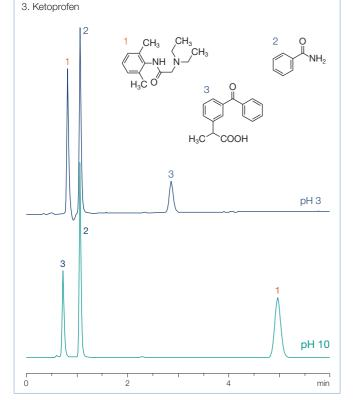
As mentioned above, pH stability of the stationary phase can be helpful for improving selectivity in method development. The following figure shows the separation of 4 basic drugs under acidic and basic conditions.
