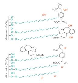
The figure above shows the extent of protonation of surface silanols and of two exemplary analytes at acidic and alkaline pH. The following graph explains the general correlation between retention and pH.
