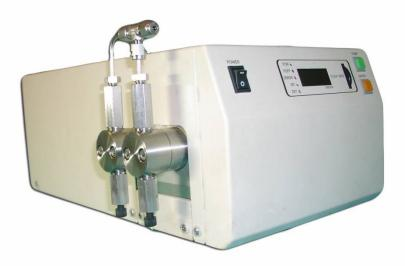
The check valves, which have been developed for high viscosity fluid delivery, has enabled our pump system to deliver high viscosity fluid with high pressure such as commercially available glycerin solution (approx. concentration 85%). Though actual flow rate is reduced by the flow resistance when inhaling the fluid, good flow rate reproducibility is obtained and efficiency of the delivery can be increased with special modifications of tubing in the inhaling side.
