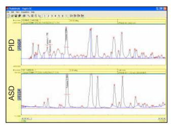
Notice the comparative chromatograms here showing the response of the PID and ASD detectors plumbed in series to an injection of 1000ppm each Heptan and Toluene. The ASD shows no response to the Heptane but good response to the Toluene.
