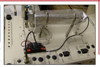
The ASD consists of a 15cm long heated tube with a mercury lamp mounted at one end and a photodiode at the other. It can be mounted on an SRI GC or on the separate Model 110 chassis which is then connected to any GC. The ASD detects only those molecules which absorb the 254nm wavelength produced by the mercury lamp. Aromatic compounds such as Benzene and Toluene absorb strongly at this wavelength while aliphatic compounds such as Hexane and Heptane do not.
