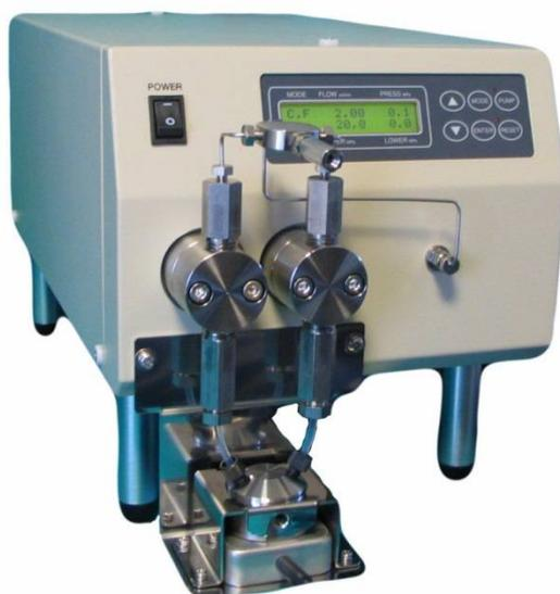
The system has been capable of delivering slurry continuously with high pressure, which was previously very difficult with the pumps available in the market. L.Tex has developed very unique structure for the check valves which has enabled the slurry to be delivered smoothly. It is required to inhale the slurry over stirring it right before the check valve depending on concentration and density of slurry. For further details, please contact us.
